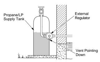
Figure 20 - External Regulator with Vent Pointing Down
